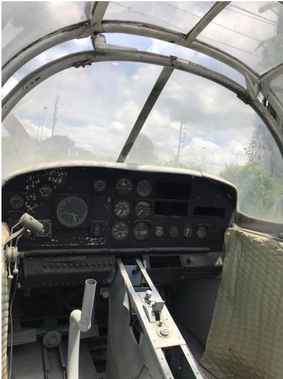
Cockpit of AESL CT-4 Airtrainer 002, showing unusual instrument layout, single controls, and original canopy. Delivered to Thai Police Aviation Division in 1973. Photo: Max Jang .....
