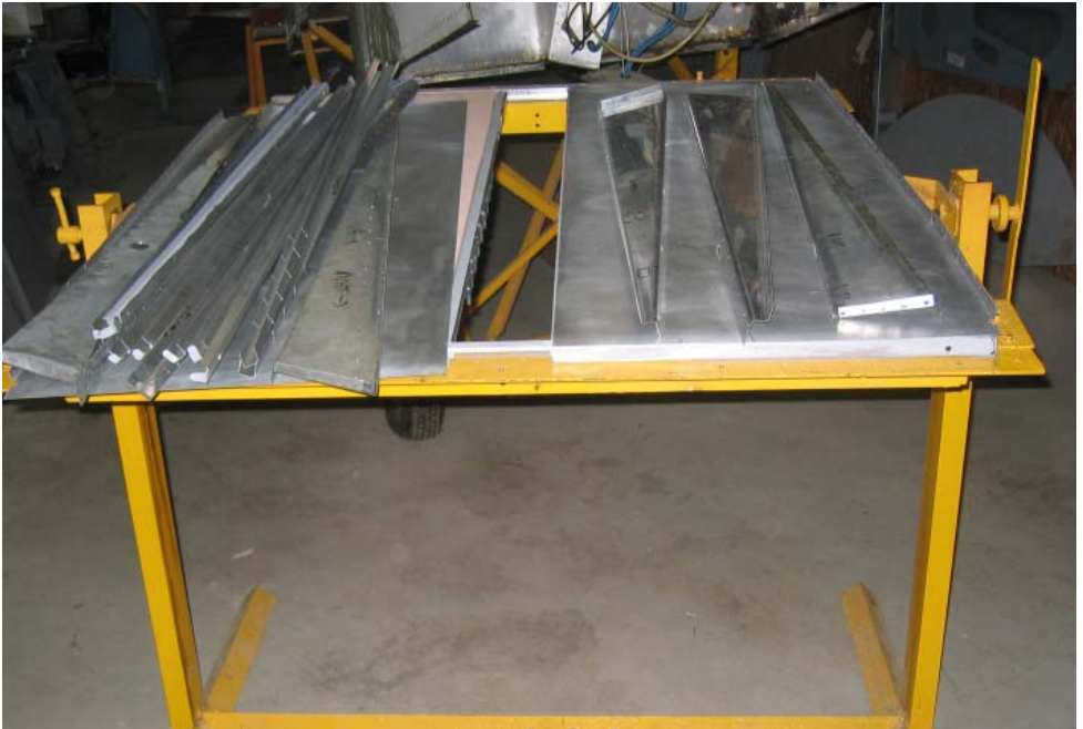
Above: Floor Pan jig. Opposite page: Some of the larger jigs.
