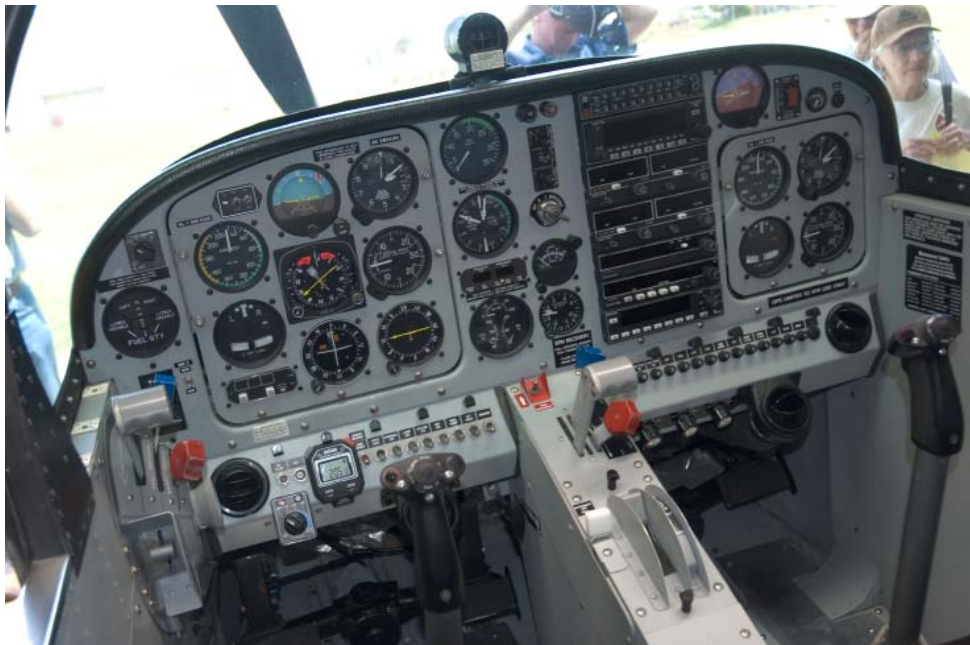
The cockpit of the CT4E, well fitted out but still with a distinctive military style. As a trainer, the right hand seat has a basic set of flight instruments.
