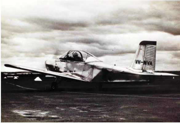
An early photo of MVA during the test program without the now distinctive dorsal fin.
